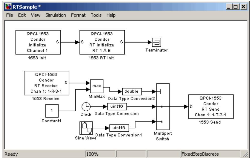
The QPCI-1553 Initialize block configures the board for Remote Terminal operation on channel 1 of the board. The QPCI-1553 RT Initialize block configures the Remote Terminal 1 to monitor buses A and B for incoming messages and configure the active transmit and receive subaddresses. The QPCI-1553 Receive and Send blocks use subaddress 3 for both transmit and receive. Note the message parameters notation 1-R-3-1 on the QPCI-1553 Receive and Send blocks. This notation has the format
