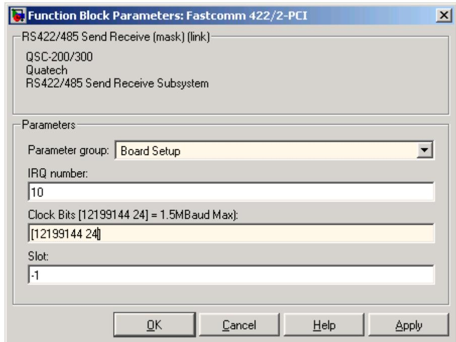
After you define a maximum baud rate, you can set a unique baud rate for each channel by choosing a different baud rate divisor for each channel. For example, you can have Channel 1 have a baud rate of 750000 (1500000/2) and Channel 2 have a baud rate of 1500000 (1500000/1). To set Channel 1 to have a baud rate of 750000, with the Fastcom 422/2-PCI Send Receive block with the **Parameter group** parameter set to Basic Setup, set
