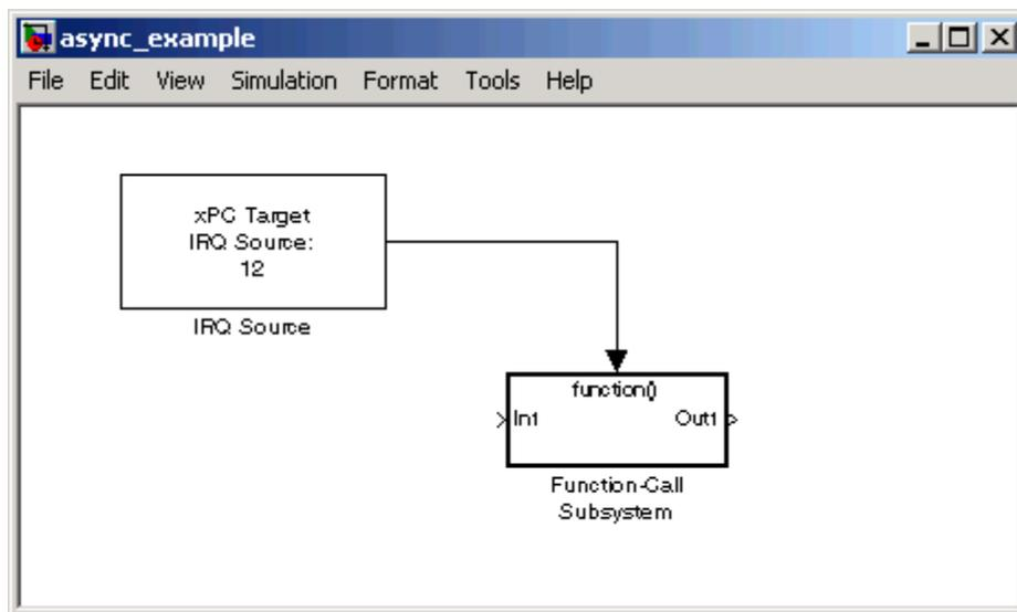
In the setup shown above, the CPU executes the contents of the Function Call-Subsystem whenever IRQ 5 occurs.
