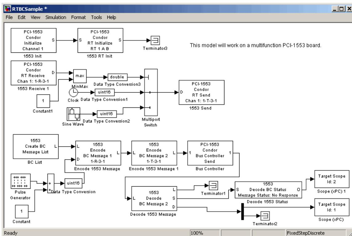
In this example, the two Encode BC Message blocks each create a message, for a total of two, in the list. The message created in the first Encode BC Message block is a receive message. Note, the direction of a message is always from the point of view of the Remote Terminal. The **Direction** parameter of the block has a value of R (BC->RT). The 1553 Encode BC Message block creates
