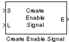
You can use a Create Enable Signal block to generate an input enable signal for A/D and D/A blocks. You can connect a signal generator to the input of the Create Enable Signal block to control the output enable port. You can then connect the output E port of the Create Enable Signal block to the input E port of an A/D or D/A block.
