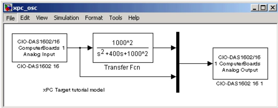
You cannot run this model unless you have the I/O board shown installed in your target PC. However, you can substitute the driver blocks for another I/O board that is installed in the target PC.
