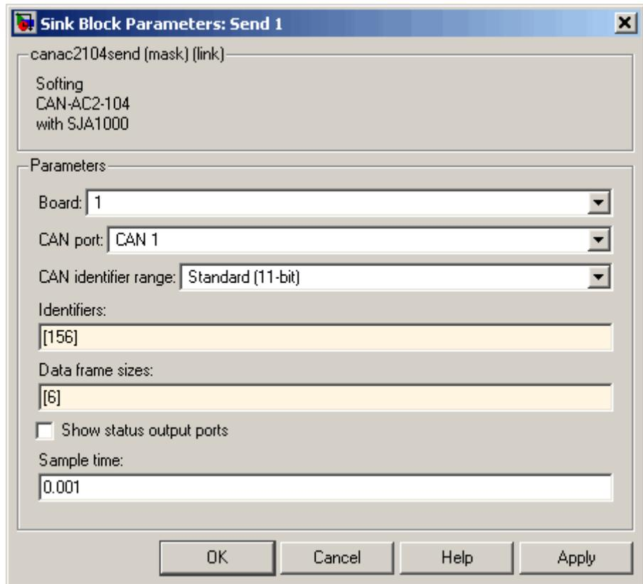
The data frame is then propagated to the CAN Send driver block and is sent as part of a CAN message having identifier 156. In the Send block's dialog box, the data frame size is defined as 6 bytes. This ensures that only the first six bytes of the incoming double value are transmitted as part of the CAN message.
