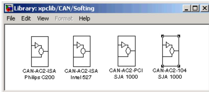
The fourth block group, CAN-AC2-104 SJA 1000, contains the three available CAN blocks: Setup, Send, and Receive, plus a FIFO Mode block, which is discussed in Chapter 6, "CAN I/O Support for FIFO".
