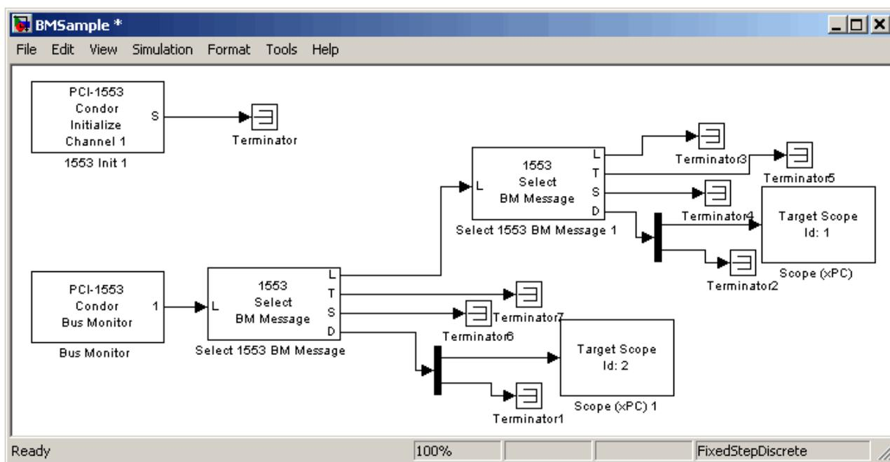
The PCI-1553 Initialize block configures a Bus Monitor on channel 1 of the board. This block also tells the board to monitor bus A. This PCI-1553 Bus Monitor block specifies a maximum of 10 messages to receive in a list.
