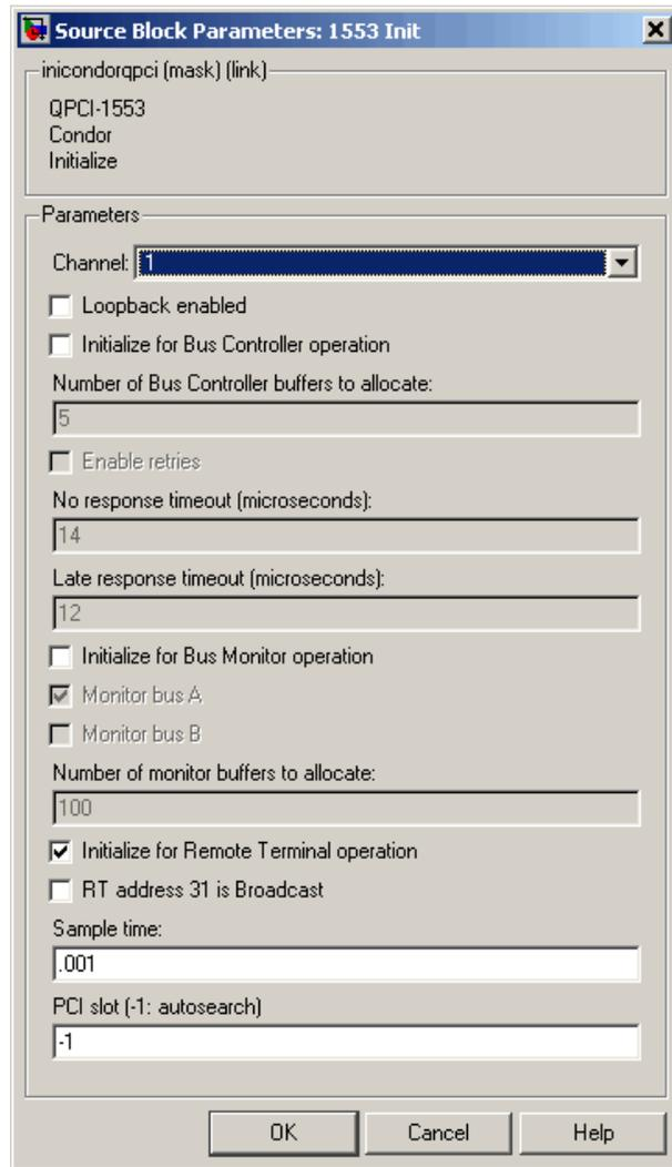
The following is a sample model of how to use the QPCI-1553 Initialize block to initialize channel 1 of a board for Remote Terminal operation. This and other examples are located in the `xpcdemos` directory. This model
