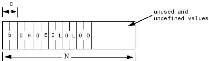
These serial blocks interpret each entry in the vector as a single character. The low-level hardware Send block writes the low-order byte of each entry to the UART. The 16- and 32-bit data types allow the embedding of any 8-bit data value, including 0. The 8-bit data type is most useful with the ASCII
