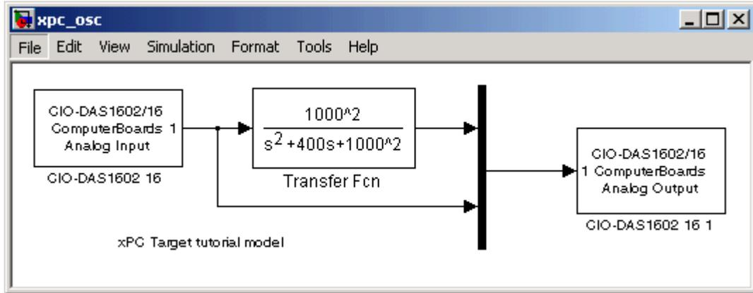
You cannot run this model unless you have the I/O board shown above installed in your target PC. However, you can substitute the driver blocks for another I/O board that is installed in the target PC.
