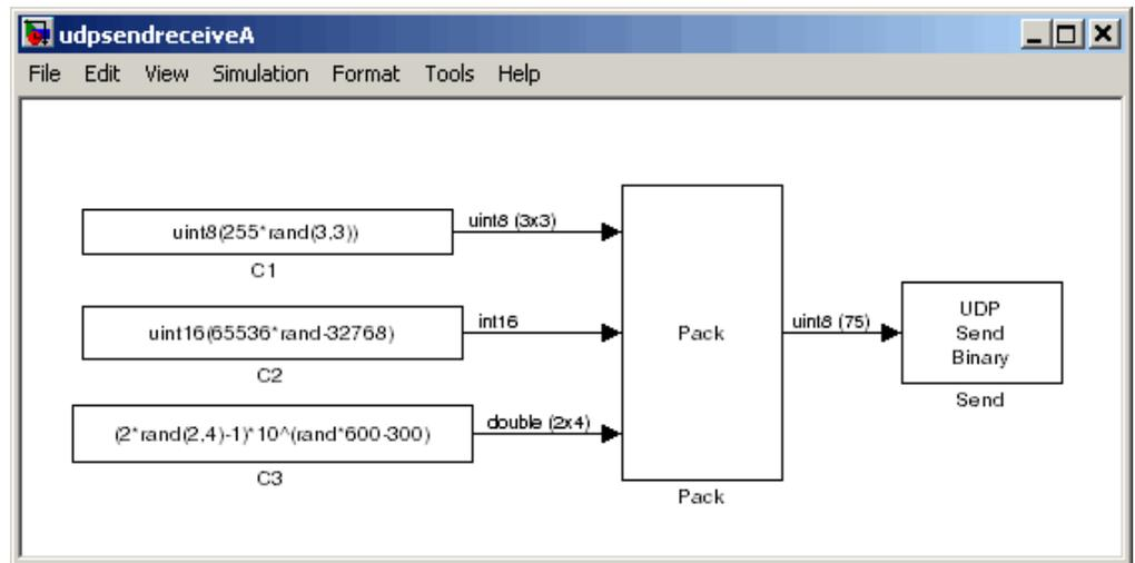
Note that the width of the UDP packet to be sent is 75 bytes. The parameters used in the Pack block are **Input port datatypes** {'uint8', 'uint16', 'double'} and **Byte Alignment 1**.
