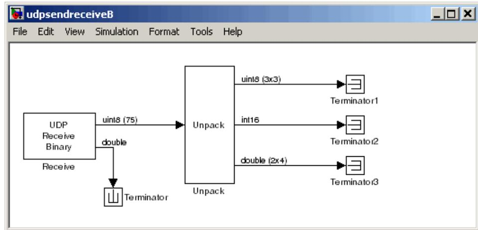
For setting up the Receive block, set **IP address to receive from** to 192.168.0.10 (the hypothetical address of the system that will run `udpreceiveB`). The **IP port to receive from** is set to 25000 (the same value as set in the Send block in `udpreceiveA`). The **Output port width** is set to 75, which is obtained from the output port width of the Pack block in `udpreceiveA`.
