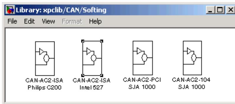
The second block, CAN-AC2-ISA Intel527, contains the three available CAN blocks: Setup, Send, and Receive.
