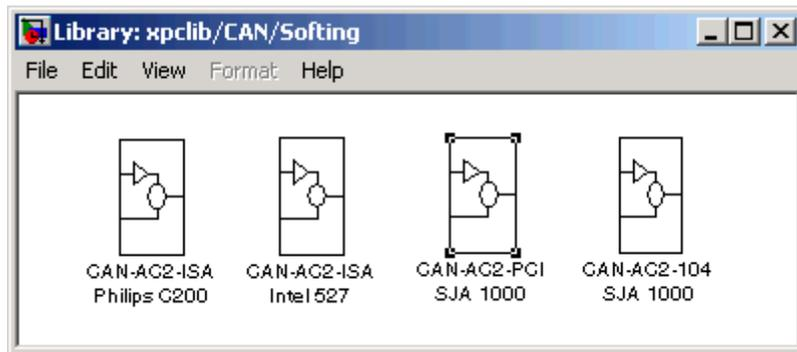
The third block group, CAN-AC2-PCI SJA 1000, contains the three available CAN blocks: Setup, Send, and Receive, plus a FIFO Mode block, which is discussed in Chapter 6, "CAN I/O Support for FIFO".
